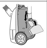
When storing the vacuum cleaner pipe and nozzle can be attached as shown in the picture.
